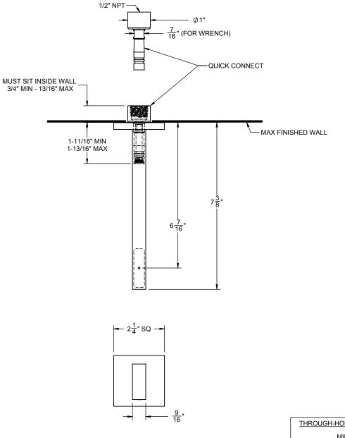
THROUGH-HOLE SPECIFICATIONS RECOMENDED Ø 1-3/8" <u>MIN</u> Ø1-1/4" SPOUT:
