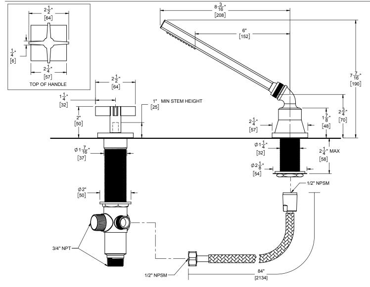
THROUGH-HOLE SPECIFICATIONS RECOMENDED <u>MAX</u> MIN SHOWER: Ø1-1/4" [32] VALVE: Ø1-7/16" [37] Ø 1-1/4" [32] Ø 1-1/2" [38] Ø1-11/16" [43] Ø1-3/4" [44]
