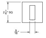
THROUGH-HOLE SPECIFICATIONS RECOMENDED Ø 1-3/8" <u>MIN</u> Ø 1-1/4" SPOUT:
