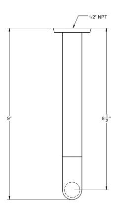
**THROUGH-HOLE SPECIFICATIONS** MIN **RECOMENDED** MAX Ø1-1/4" Ø1-3/8" Ø1-9/16"
