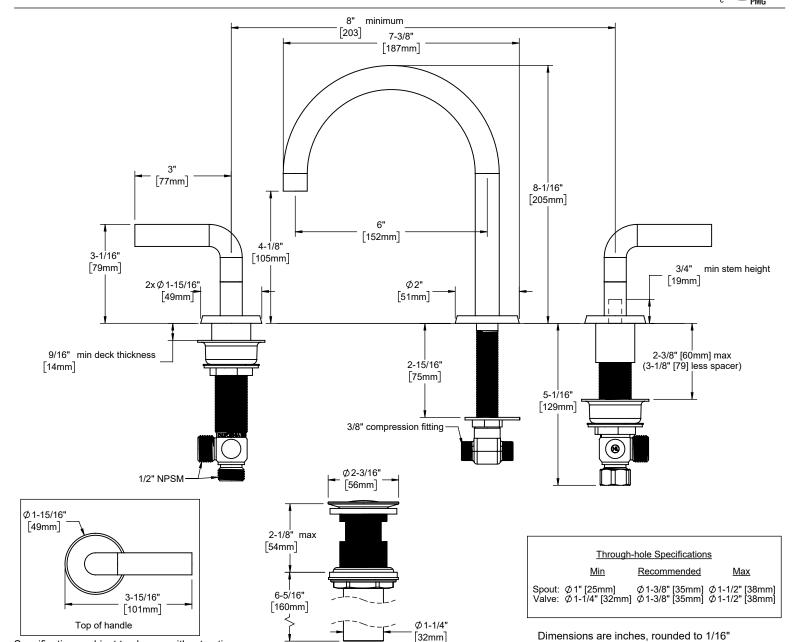
[Dimensions in brackets are mm, rounded to 1mm]
